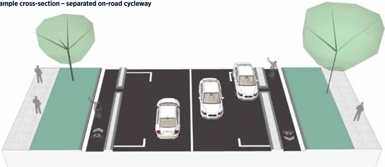
Example cross-section – separated cycleway at footpath level
